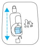
Move lock control up to engage the lock. Move control down to disengage childproof locks.
